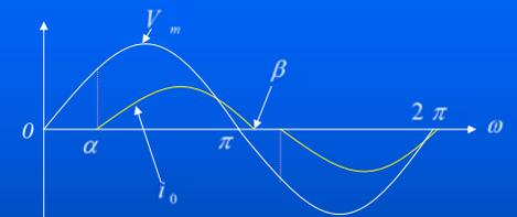
$$i(\omega t) = \begin{cases} \frac{V_m}{Z} \left[ \sin(\omega t - \theta) + \sin(\alpha - \theta) \cdot e^{-\frac{(\alpha - \omega t)R}{\omega L}} \right] & \text{at } \alpha \leq \omega t \leq \beta \\ 0 & \text{otherwise} \end{cases}$$
