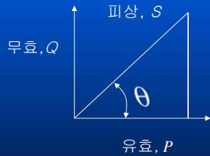
$$pf = \frac{P}{S} = \frac{V_{o,rms}}{V_{s,rms}}$$
