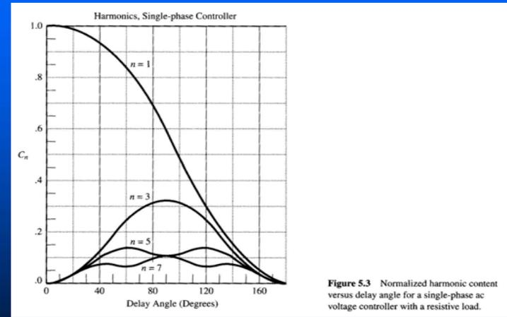
Figure 5.3 Normalized harmonic content versus delay angle for a single-phase ac voltage controller with a resistive load.
