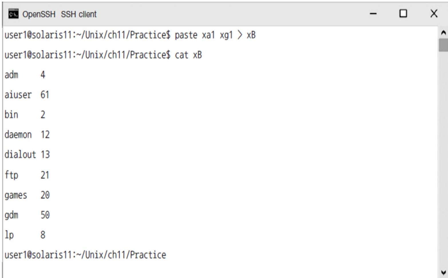
A terminal window titled "OpenSSH SSH client" showing a user performing a file concatenation task. The user runs the command "paste xa1 xg1 > xB" to combine two files into a new one. Then, they run "cat xB" to display the contents of the new file, which shows a list of system users and their IDs.
